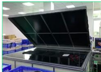
EL testing for foldable solar panel
